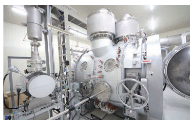
A huge silencer at the top catches the eye. The sub-chamber is on the left.
