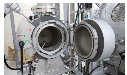
The combustion of the fuel used in the experiment is checked in the sub-chamber.
